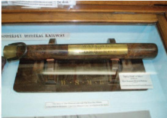
This type of staff was used on all single line railways. It was given to the driver by the signalman, and it allowed the driver to take the train along a length of single line, knowing that he would not collide with a train coming the other way, as there was only one staff on each length of line.
